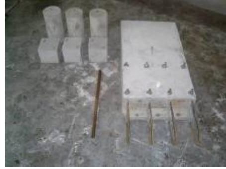
Fig. 6. Concrete and steel samples
