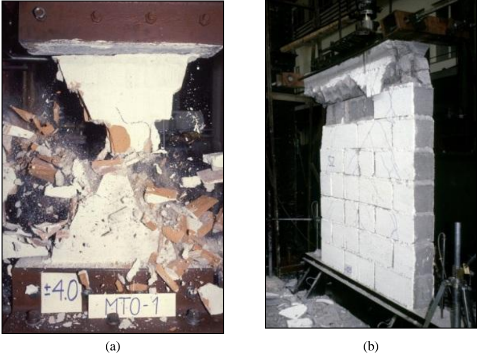
Figure 5. Brittle shear failure of a highly stressed unreinforced masonry wall (a) and (b) brittle failure of a complete course of concrete hollow blocks which prevented the activation of reinforcement
