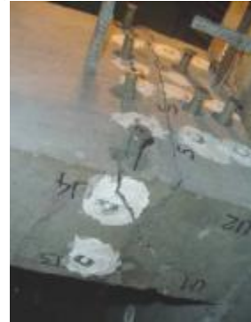
Fig. 15. Failure mechanism of precast specimens: A) Crack pattern; B) Precast specimens by yielding of reinforcement
