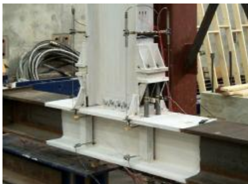
Figure 6. Integral beam-column connection investigated by DesRoches and Ocel, [13]
