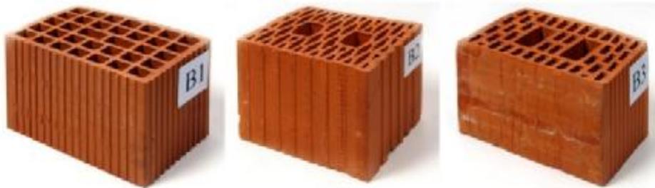
Figure 6. Typical hollow clay blocks tested in the experimental campaign [18]
